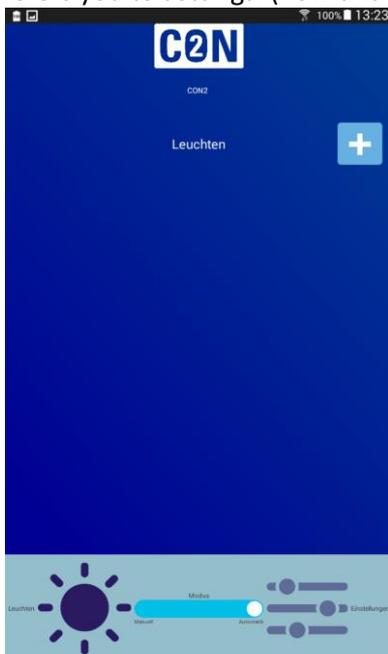
5. After pressing the plus button new lights can be assigned to slot's. Then one can choose the programmed luminaries in the main menu.
